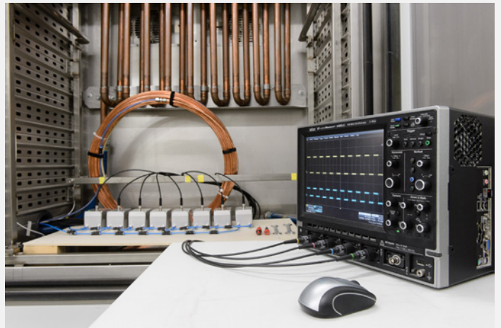
Fig. 4: Calibration of multiple gas quality sensors [6]
